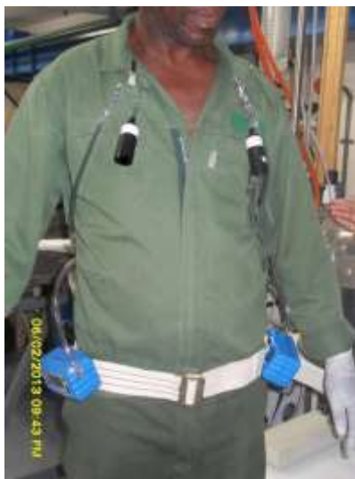
Figure 3: A worker with personal sampling train attached.
