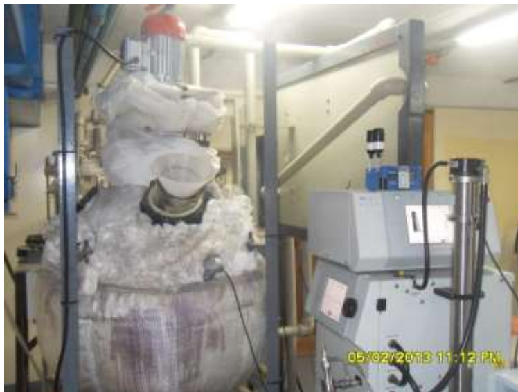
Figure 2: Chemical reactor with real –time measurement instruments, SMPS and APS, with occupational hygiene pumps on top.
