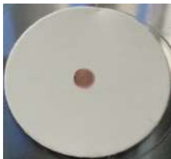
Figure 4: Carbon coated TEM copper grid on a MCE filter
