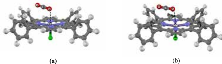
Figure 1. Optimized structure for (a) CO 2 @ Fe-PCN-222 and (b) CO 2 @ Mn-PCN-222 with M06-L functional.
