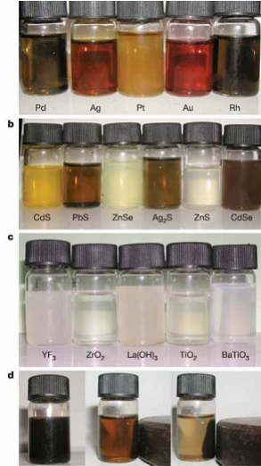
Figure 4 | Cyclohexane solutions of nanoparticles with a typical concentration of 2%. a-d, Cyclohexane solutions of noble metal (a), semiconductors (b), rare earth fluorescence (c) and magnetic nanocrystals (d). d, The separation of \text{CoFe}_2\text{O}_4 nanocrystals from the bulky solution by magnetic force.
