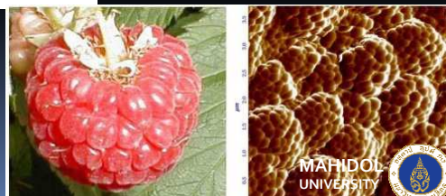
Raspberry-like particles made of silica spheres bonded to an epoxy-based polymer film.
